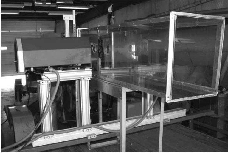
FIG. 1— Sympatec system positioned on both side of the high speed tunnel with the tunnel outlet on the right side of the picture.
